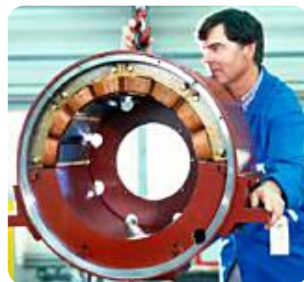
View of a 400 mm diameter radial magnetic bearing
