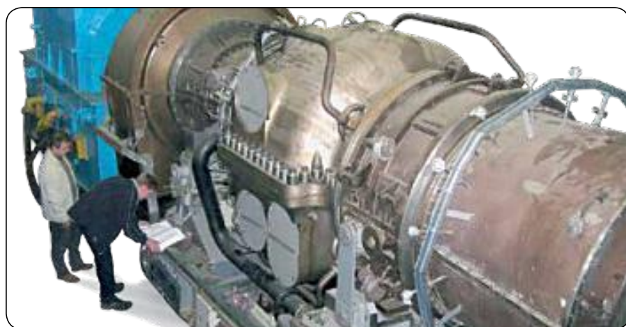
The gas turbine drives the electric generator and provides heat (hot water) in a cogeneration plant
